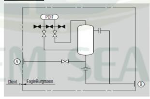
P&ID for LSA60000 -A4 Leakage collection system
